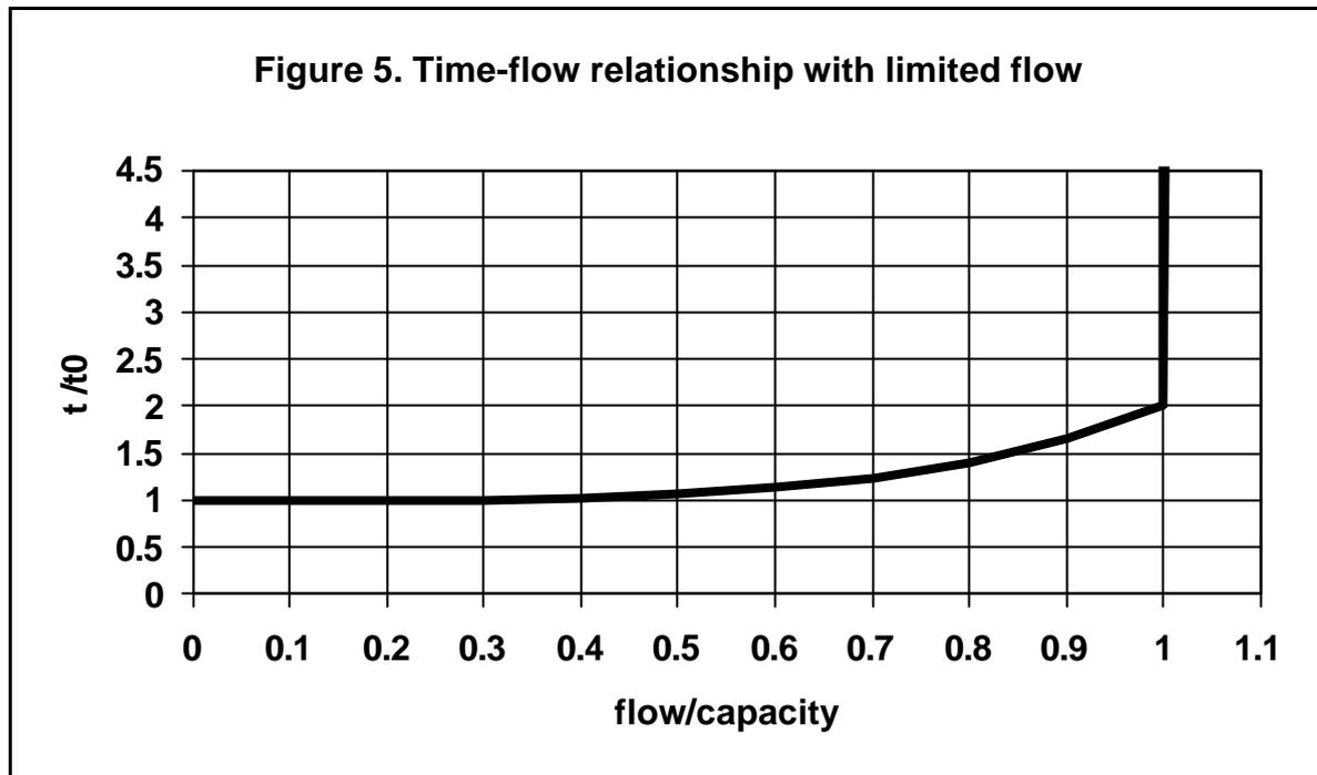
The UBA incorporates a gravity model with an upper constraint for the time budget [16]. If roadways are improved, this constraint doesn't get effective at all. Thus the induced travel is taken into account only roughly.
